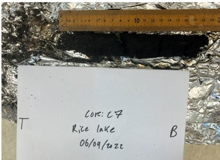
Figure 2. Example sample core from sampling location C7 before drying, with no clearly identifiable sedimentary horizons within the core.
